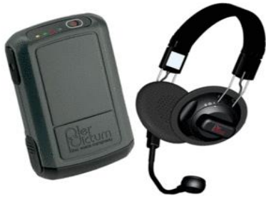
Figure 3 - Pick by voice technology - equipment for the picker [14]
