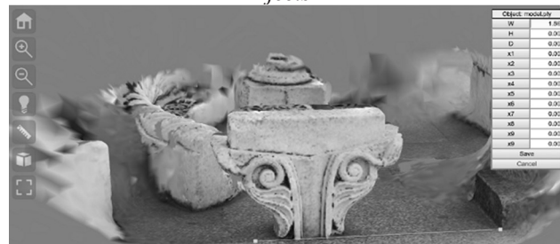
Fig. 3. Web based measurement system for 3D objects
